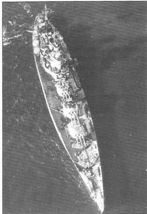
A British Nelson-class battleship. The unusual arrangement of turrets was employed to achieve maximum firepower while staying within treaty weight limits.
