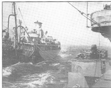
An oiler refuels a warship. The Germans depended on such mid-ocean refueling to keep their raiders under way.
