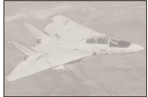
Figure 1-1: An F-14 in a high energy state with wings swept back for speed.
