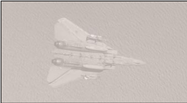
Figure 3-4: This pilot is pulling some heavy G's in this 900 left bank. With his wings swept full aft, you can get some indication of his energy state.
