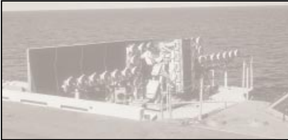
Figure 3-12: The "meatball" is a visual landing aid which helps pilots assume the proper 3° glideslope during the final approach leg of the traffic pattern.
